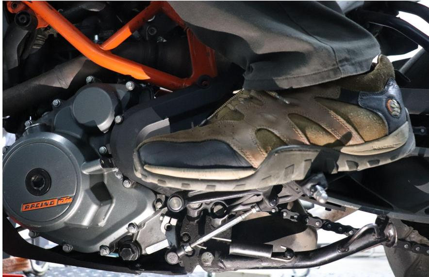
2.3. Move the shift lever like shifting up a gear, like going from 1st to 2nd, or 2nd to 3rd, etc.
