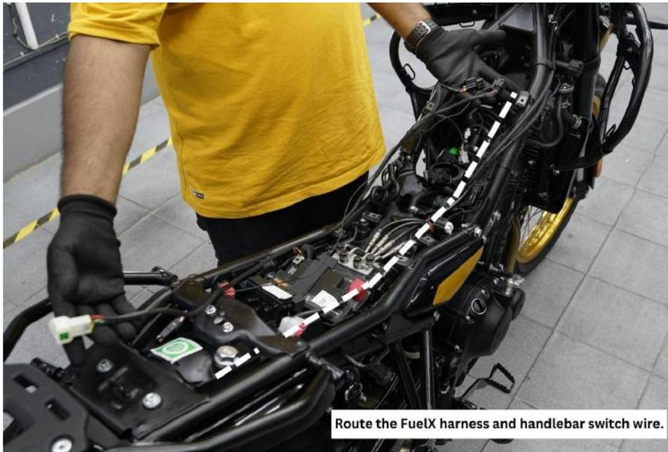
Route the FuelX harness and handlebar switch wire.
