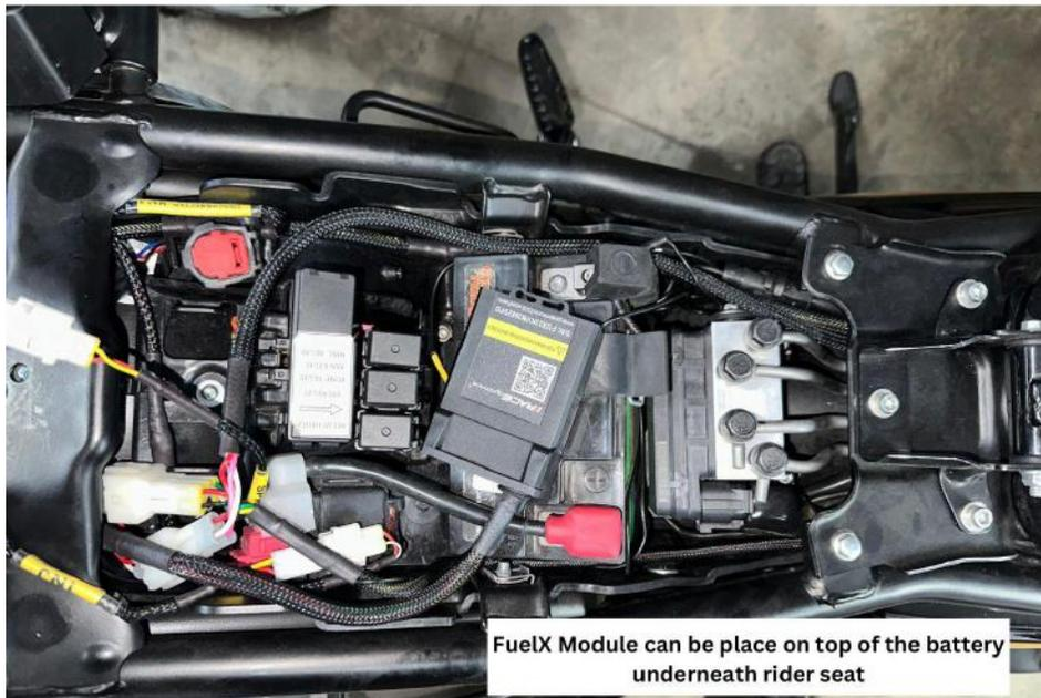
FuelX Module can be place on top of the battery underneath rider seat
