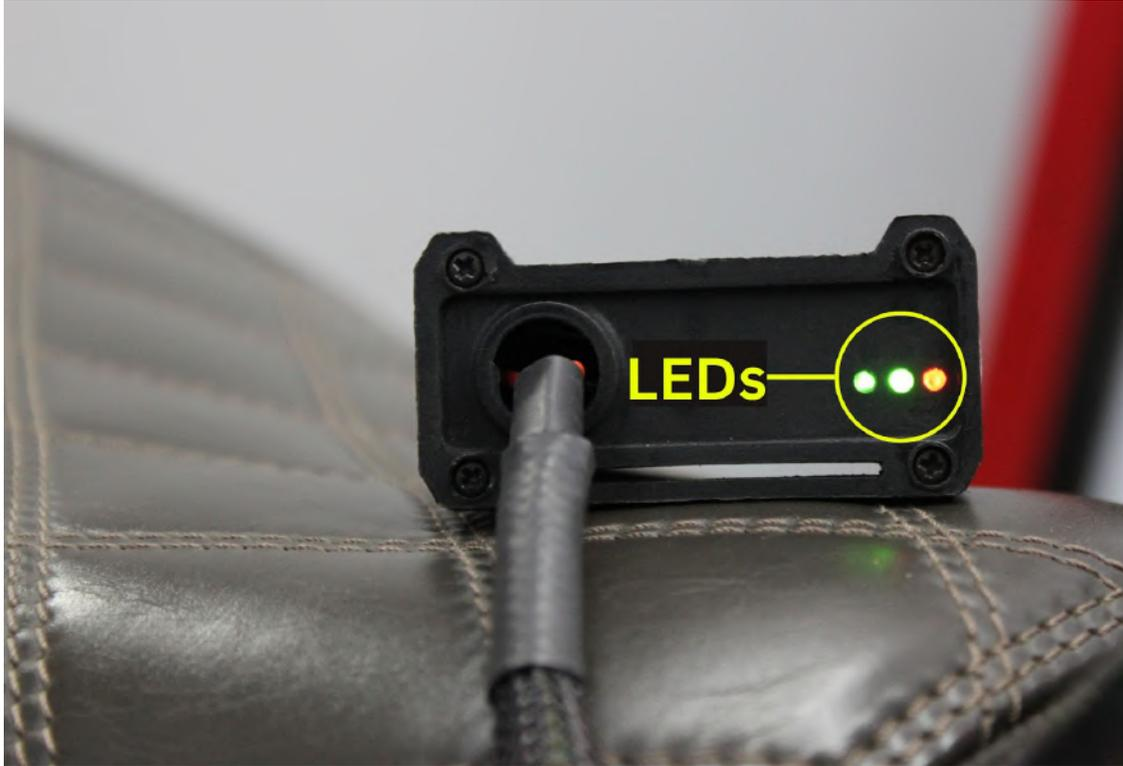
The blinking of the **Red LED** indicates that the Map on the FuelX is being activated. The Red LED starts blinking after the key and the kill switch are on.
